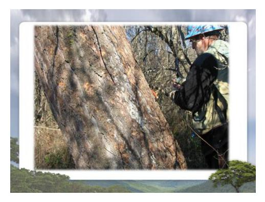
Here is the handle that you actually turn, it screws into the tree, and here is the actual boring part that will go into the tree. The alignment here is that Ted is actually trying to aim that bore right into the center of the tree to try to encompass all the rings to get an accurate core date. Here we see that the handle is screwed all the way into the tree. It was almost at the limit of his tree bore. Then what he is doing is sliding out the core sample here.
