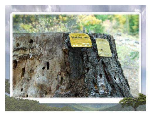
Going to the next slide, let us talk about the order of BT marks. These BT marks are always read sideways from the top to the bottom of the tree. Here I have an example that was sawed off a tree that when 109 I am talking about marks being read sideways. The top of the tree would be up here, the bottom
