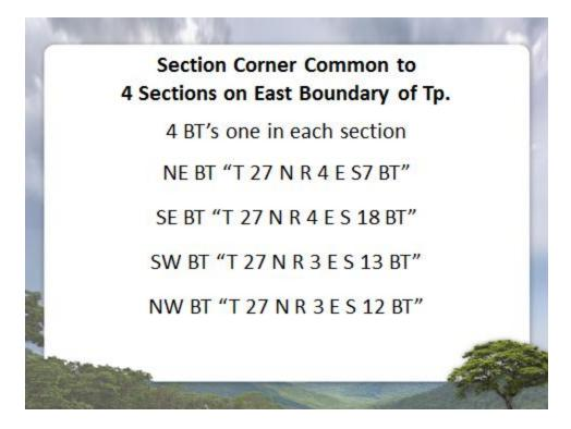
Since it is common to four sections it requires four bearing trees. One in each section. As you can see here that I have chosen the corners of sections 7, 12, 13 and 18. Since we are on the boundary the east boundary of the township, we have two different ranges that are involved. So the north east and south east trees are going to reflect the fact that they are in range 4 E, and Westerly bearing trees in the south west and north west are going to reflect the fact that they are in range 3 East.
