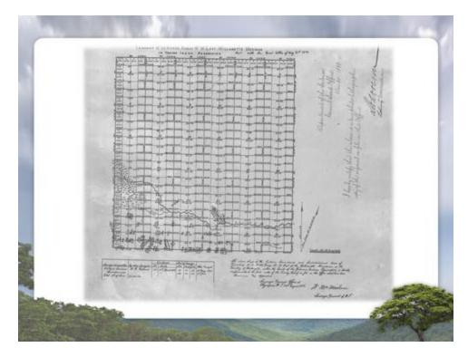
Let us focus in here on Section 8. Here we see in Section eight, while we have three lines typical of a three mile survey done east to west, where the center of the section was set at midpoint, the center south 1/16th set at midpoint east west and the center north 1/16<sup>th</sup> set at midpoint east west. None of the north south lines were surveyed.
