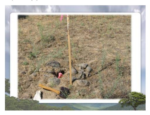
The legal description for this corner, the description given in the GLO notes for this corner was that it was a wood post within a mound of stone. What's interesting is that the center of this ring of stones, you can see the rings and how the stones are embedded around forming a circular ring that the actual center of this although we did not find any remains of the wood post, the center was very soft. As if the post had been pulled out and filled in with sand over the years.
