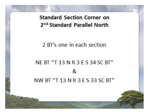
This will be a corner that is common to two sections, so we want two BTs, one in each section. Now the second standard parallel north would be the south boundary of township thirteen north. So this bearing tree to the northeast in section thirty-four would read T 13 N R 3 E S 34 SC (since it is a standard corner) BT. And the other bearing tree to the north west in section 33 of course would have the Township 13 North Range 3 East Section 33 SC for standard corner and BT.
