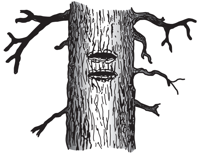
Figure 3-53. Hack marks on a line tree.
